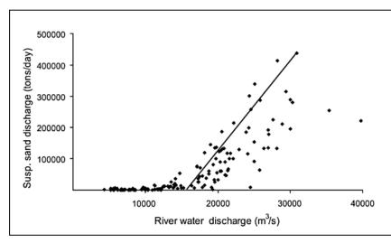
Figure 1: From Nittrouer et al, 2008. Plot showing a considerable flow and sediment discharge hysteresis. Suspended sand discharge is strongly related to the presence of large dunes. The vast majority of sediment movement events occur above a flow threshold of ~16,000m<sup>3</sup>s<sup>-1</sup> because this is where large bedforms start to form.
