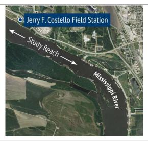
Figure 3: Field site. The USGS field station is located just above the confluence with the Missouri River, North of the city of St. Louis. The survey reach is a section of straight sandy bed channel ~ 10 km long and 1 km wide with mean annual depths ~12m.
