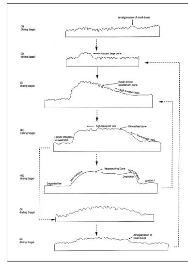
Figure 2: From Carling et al, 2000. Conceptual diagram displaying dune morphology during rising and falling legs of a flood wave. Various scales of bed features form and move downstream depositing cross strata. Such diagrams would be considerably improved by very high resolution measurements of the cross strata and bed morphology through a flood wave, providing event scale preservation potential data.
